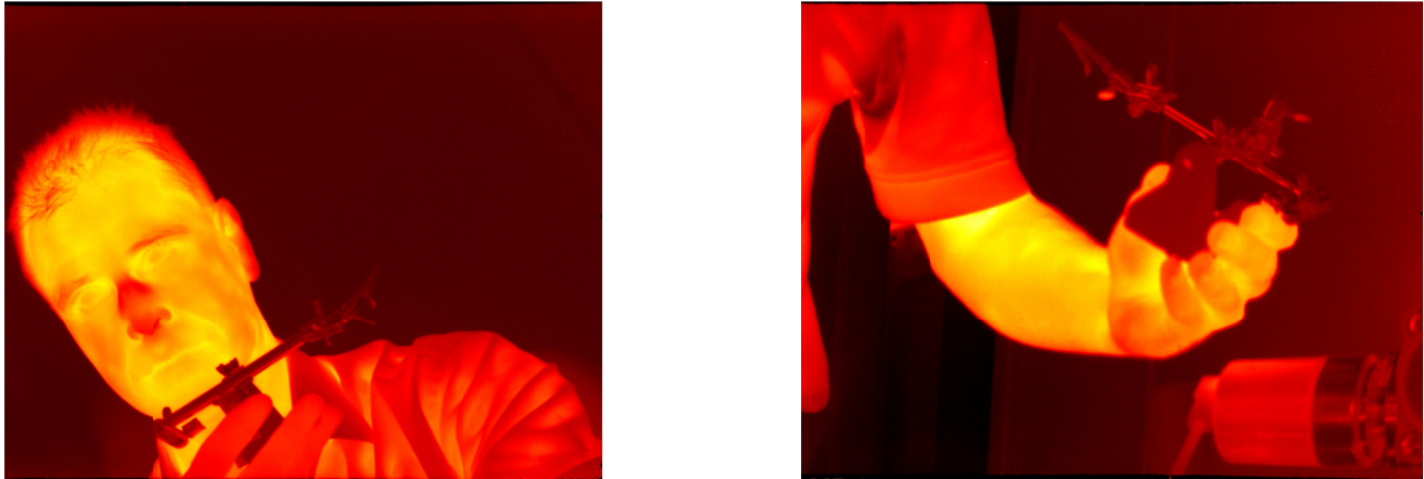
Figure 8 Images taken at 90 K with a 640 by 512 pixel, 15 \mu\text{m} pitch focal plane array processed from Design A material.
