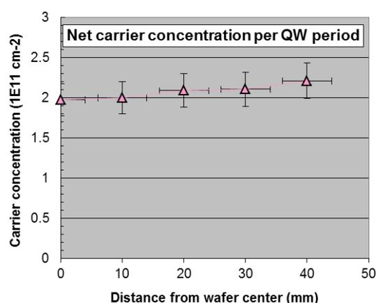
Figure 2. Net carrier concentration over the radius of a 4” wafer at 5 different positions
