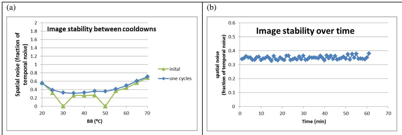
Figure 9. (a) Spatial noise versus black body temperature showing correctability and image stability after one temperature cycle (2-point corrections were performed at 30 °C and 50 °C). (b) Spatial noise versus time. 2-point correction performed with the same gain and offset map derived from measurements at t = 0
