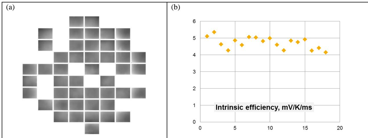
Figure 7. (a) reconstructed wafer map, each sub image represents the field of view corrected responsivity, the grey scale corresponds to  $\pm 10\%$  of the mean image value (b) variation of the intrinsic detector efficiency of detectors from the same wafer
