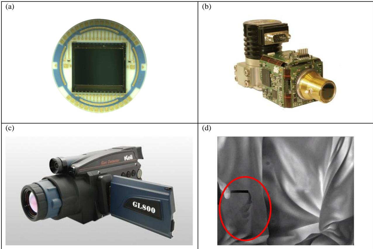
Figure 14. (a) Photo of a IRnova 10.55 FPA on ceramic carrier (b) Photo of IRnova 10.55 DDCA (c) Keii Camera with an IRnova 10.55 DDCA inside, Courtesy of Keii ) (d) Image with an IRnova-ER10.55 FPA at 56 K with escaping Sulphur Hexafluoride in the circle
