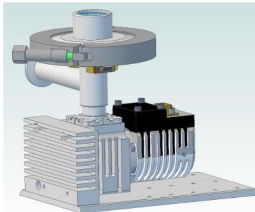
Figure 6. Test Dewar used for the radiometric testing of FPAs
