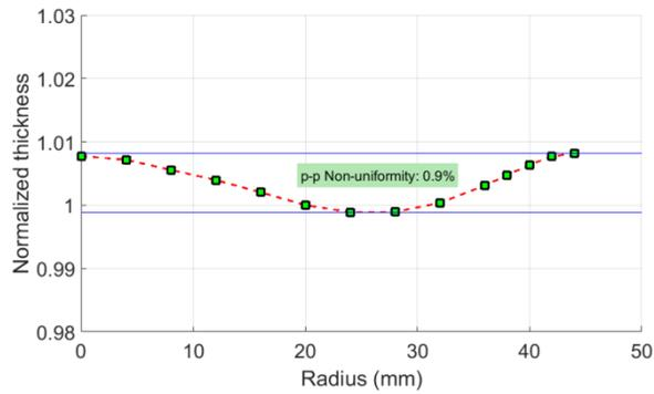
Figure 3. Normalized thickness uniformity of a MQW-structure measured radially with XRD
