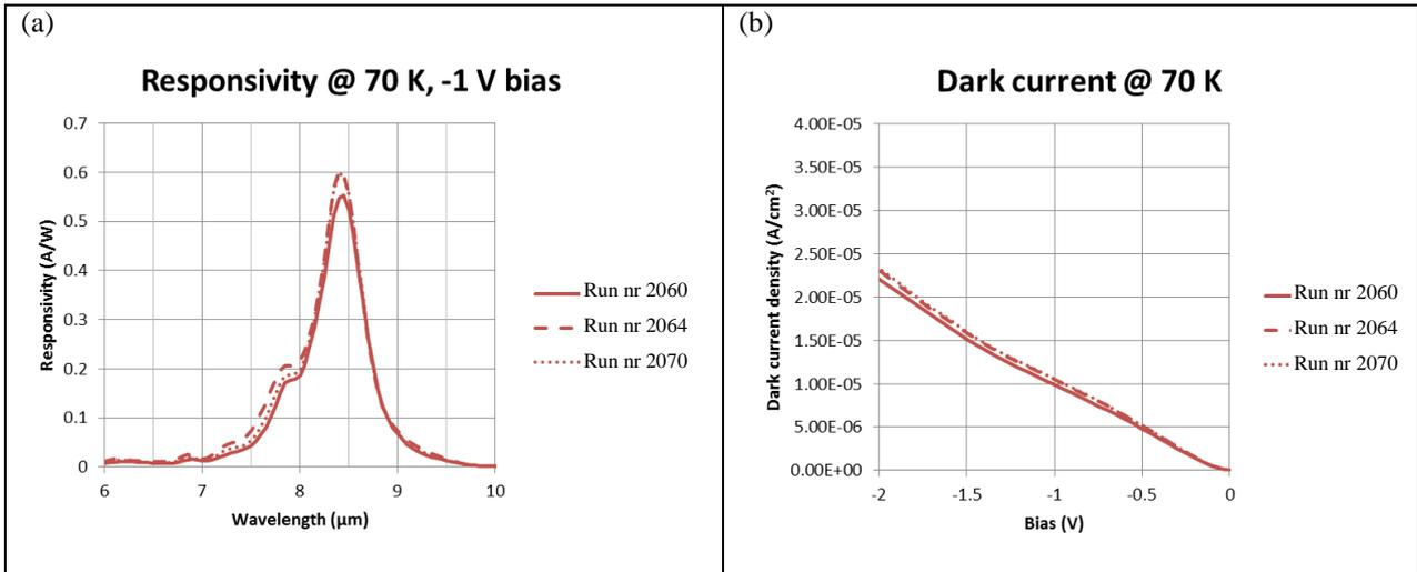
Figure 5. (a) Responsivity and (b) Dark current density for three different wafers of the same EPI campaign, measured at 70 K. Run numbers 2060, 2064 and 2070 are respectively from the beginning, middle and end of the EPI campaign.
