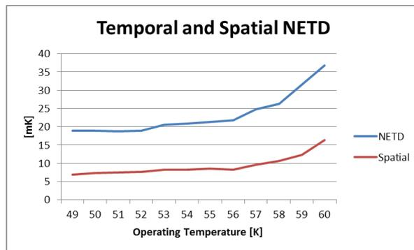
Figure 12. Temperature dependence of the temporal and spatial NETD from 49 to 60 K
