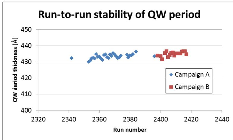
Figure 4. Thickness deviation of one period of an MQW-structure from run to run
