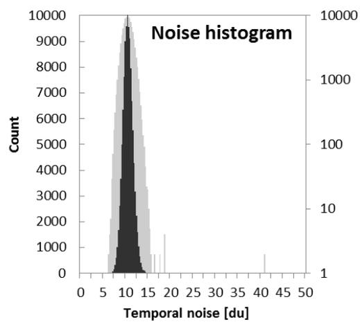
Figure 8. Distribution of the temporal noise of all pixels of an array when looking at a blackbody of 30 °C. black: linear scale, grey: log scale
