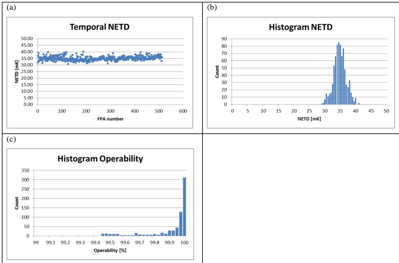
Figure 10. (a) Temporal NETD for more than 500 production quality FPAs (b) Distribution of the NETD from the same population (c) Distribution of the operability; were a pixel is declared as non-operating pixel according to definition in Table 2
