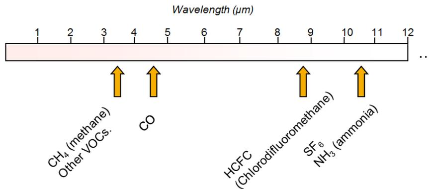
Figure 11. Absorption peaks of some different gases
