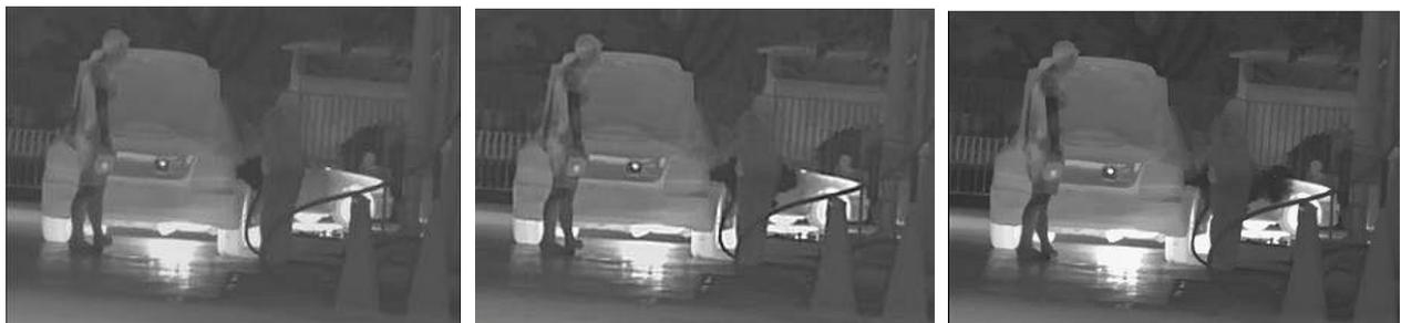
**Figure 5.** Detection of methane gas with a VOC detector, taken with an IR camera with an IRnova 320 × 256 VOC FPA inside (mounted in an IDCA). When removing the nozzle, a methane cloud (seen as a black cloud in the images) is seen around the nozzle.
