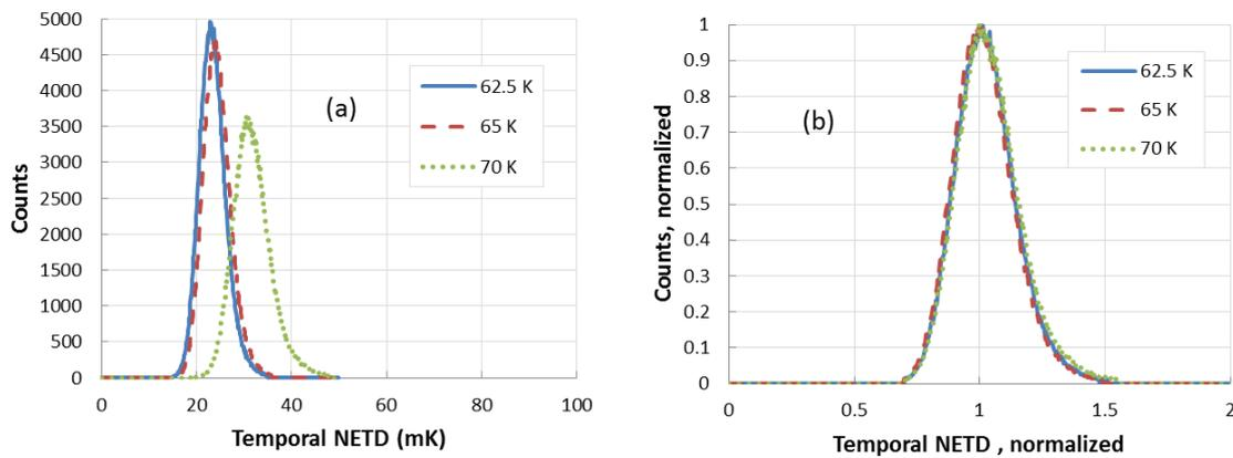
Figure 8. NETD histogram (a) and NETD histogram normalized w.r.t. counts and median value (b) for different FPA temperatures.
