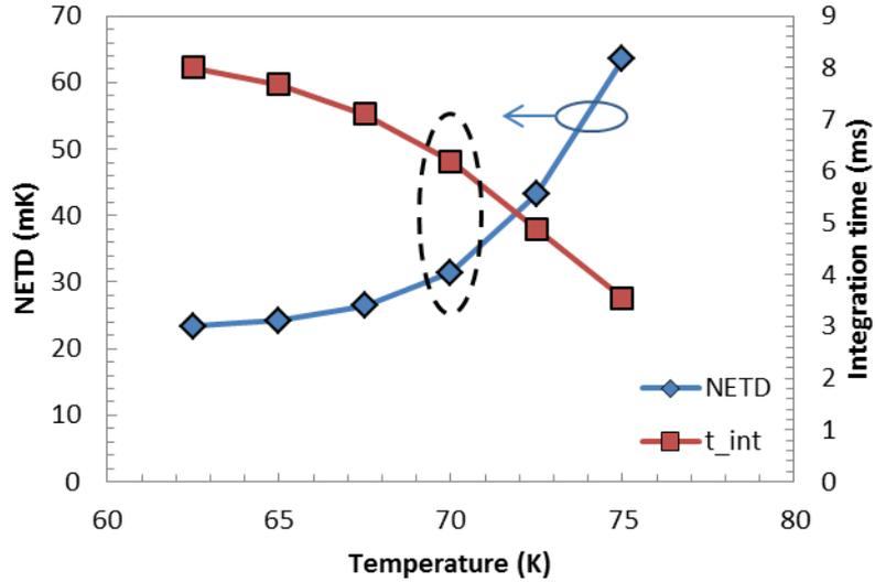
Figure 7. Recorded detector performance with a temperature sweep from 62.5K to 75K
