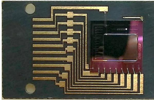
Figure 1. The test cell consists of a part of a thinned-down detector array that is flip-chip hybridized to a silicon fan-out chip. The latter is glued and wire-bonded onto a carrier which mates to the cryogenic electro-optical measurement setup.
