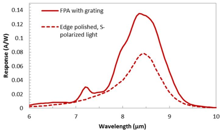
Figure 5. Response spectrum comparison for pixels with and without grating dots, the gratings of the FPA enhances light coupling, resulting in higher response. Peak wavelength is close to 8.5 μm in both cases.
