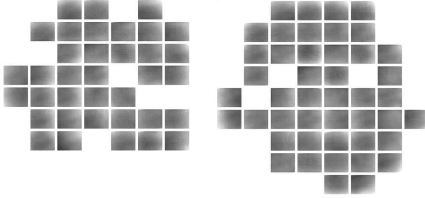
Figure 2. Gain maps (cos4 corrected; grey scale  $\pm 10\%$  of average value) of last 2 wafers from SF<sub>6</sub> production. Few arrays can be seen missing from the wafer map, some arrays are diced for the fabrication of test cells, few are diced to check the process uniformity over the wafer and remaining lost arrays exhibited defects introduced due to particles during the wafer process.
