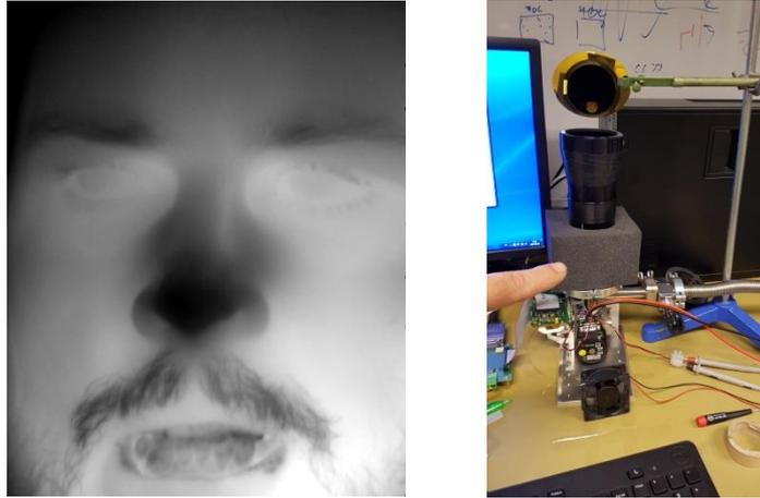
Figure 9. One frame of a video image taken with 640×512 QWIP FPA with @ 15μm pixel pitch. The image is taken with a very basic setup as shown in the adjoining figure
