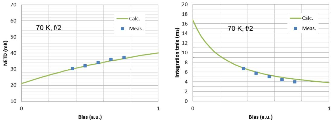
Figure 4. Simulated and measured FPA NETD (left) and integration time (right). A very good agreement is obtained between simulation and measurement without any fitting parameters
