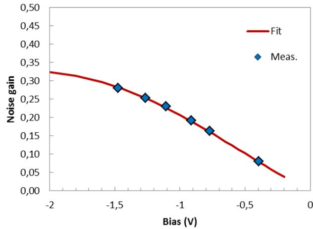
Figure 3. Noise gain of the QWIP structure as obtained on a single-pixel sample under dark conditions at 77 K by dividing the current noise squared by the current:  $G = n_I^2 / 4eI$
