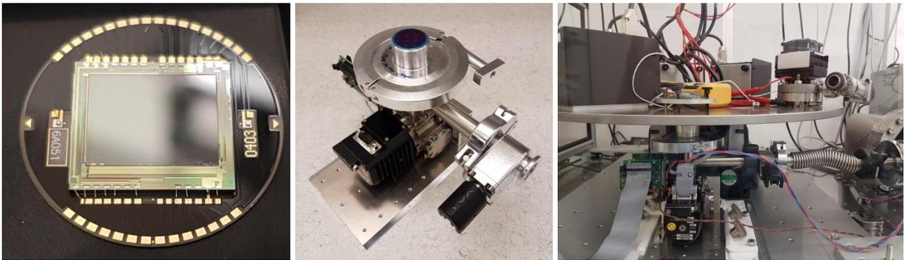
Figure 6. General view of a) an FPA mounted on the ceramic carrier, b) test vessel for FPA characterization, c) station for characterization of FPA.
