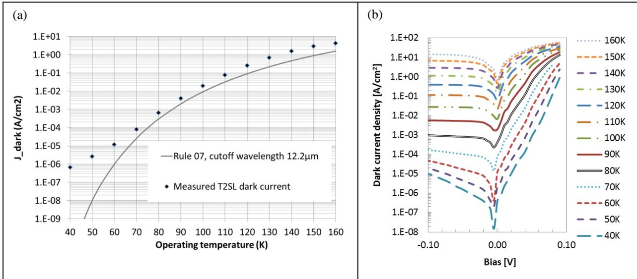
**Figure 7.** Dark current of a 12.2  $\mu\text{m}$  T2SL LWIR detector (a) Comparison of dark current density at -0.05 V with Rule07 shows that the dark current density is only 2-3 times higher than Rule07 at temperatures  $\geq 80 \text{ K}$  (b) Dark current density vs applied bias in the temperature range 40 K – 160 K for a 90  $\mu\text{m} \times 90 \mu\text{m}$  single pixel device.
