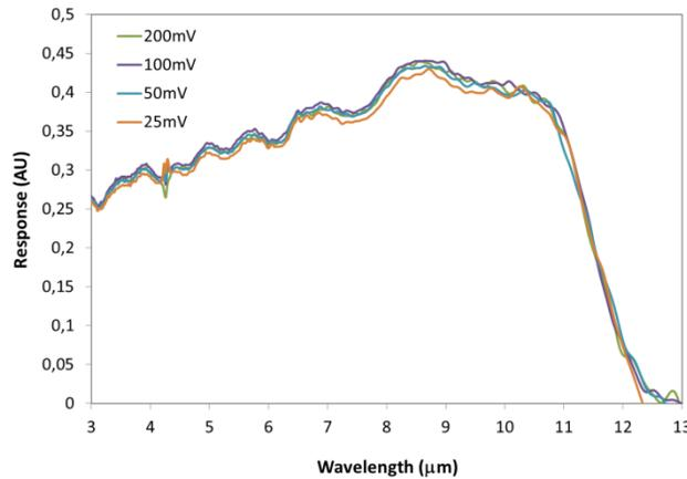
**Figure 8.** Response of the 12.2  $\mu\text{m}$  T2SL LWIR detector operated at 77K.
