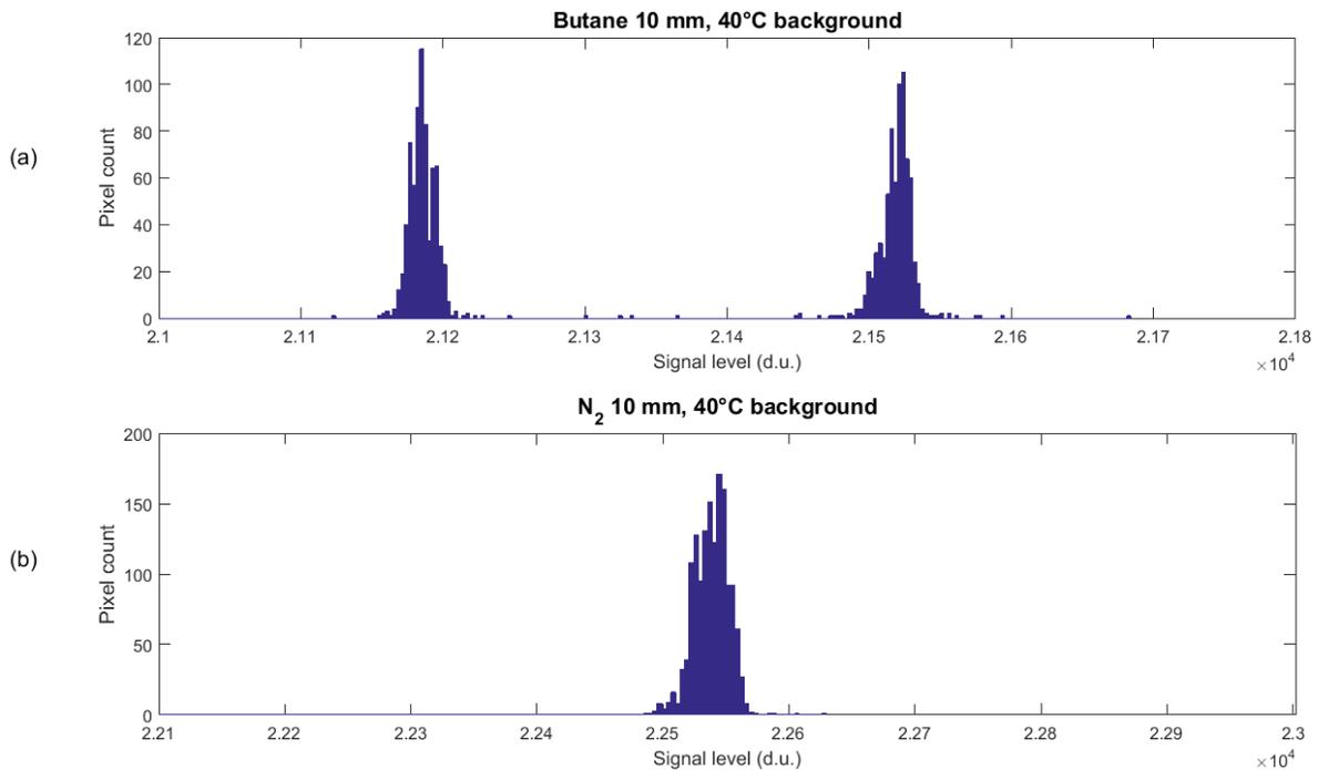
**Figure 5.** (a) Distribution of pixel values with butane gas present (b) Distribution of pixel values with  $N_2$  gas present. In both cases a  $40^\circ\text{C}$  black body source was imaged.
