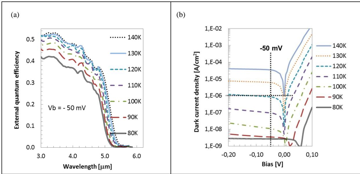
**Figure 2.** (a) Detector quantum efficiency at an applied bias of -50 mV and (b) dark current density in the temperature range  $T = 80 - 140$  K
