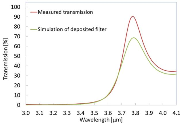
**Figure 3.** Measured transmission spectra of the pixel filter deposited on the array compared to the fitted calculation.
