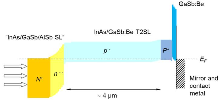
**Figure 1.** Double heterostructure (DH) detector design used in IRnova's detectors
