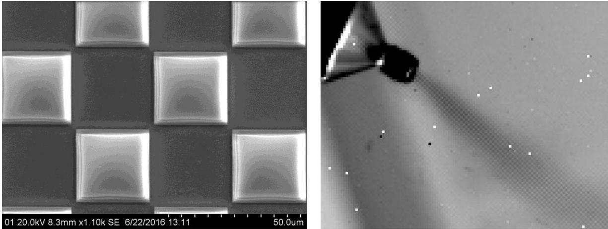
**Figure 4.** (a) SEM image showing the checker board patterned pixel filters (b) Image of butane gas flowing from a bottle, showing the checkered pattern in the image where the gas affects the signal of the filtered and unfiltered pixels differently.
