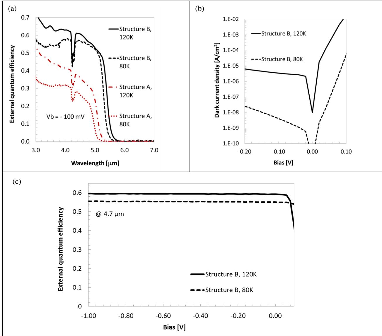
**Figure 6.** (a) Comparison of the detector quantum efficiencies for Structure A and Structure B at an applied bias of -100 mV and (b) Dark current densities for the Structure B at T = 80 K and 120 K (c) Bias dependence of the detector quantum efficiency of structure B (at 4.7 μm).
