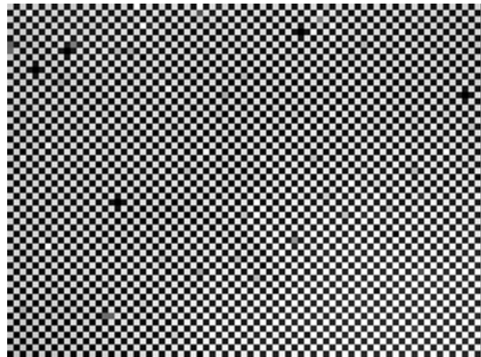
Figure 3.4. Image from FPA with 40 °C blackbody and butane gas present (RT)
