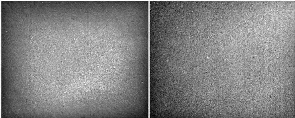
Figure 5. Gain correction map for two different detectors at 70 K; grey scale is +/- 5% of average.
