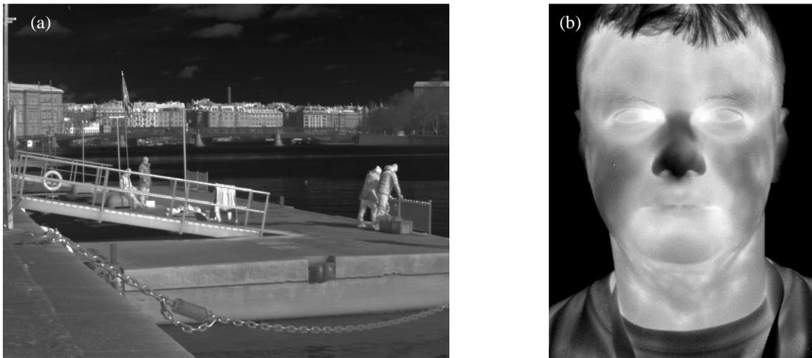
**Figure 14.** IRnova640 MW performance demonstration. (a) Stockholm quayside at ca. 0 °C outdoor temperature; 80 K detector temperature., (b) One author in room temperature environment; 120 K detector temperature, 10 ms integration time, F/4 aperture.
