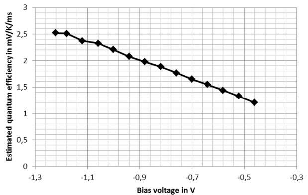
**Figure 7** The estimated collection efficiency given in mV/K/ms versus the bias voltage.
