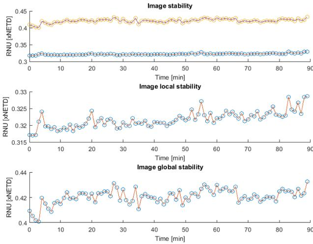
**Figure 8.** Residual non-uniformity normalized by the NETD for a measurement cycle of 90 minutes. From top to bottom: local and global image stability in the same scale; local stability; global stability.
