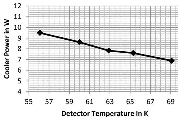
**Figure 12.** Power consumption of an IDDCA module in steady state versus detector temperature.
