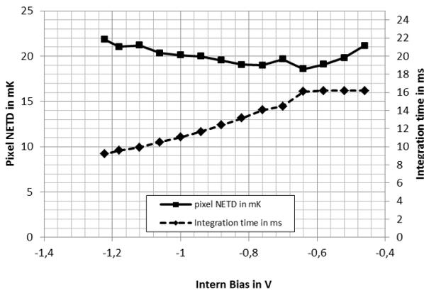
**Figure 6** Pixel NETD at 65K K as function of the bias voltage; integration time is limited for 60 Hz frame rate.
