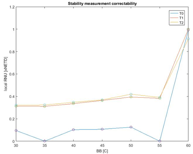
**Figure 9.** Local RNU is given normalized by the NETD showing the NUC stability for three cooling down cycles.
