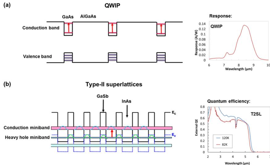
**Figure 1.** The two different detector technologies used at IRnova: (a) QWIP detectors which are based on intersubband transitions which generate narrow band response (b) T2SL detectors which are based on interband transitions with broadband response.
