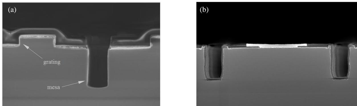
**Figure 2:** SEM cross-section images of a (a) QWIP pixel (b) T2SL pixel
