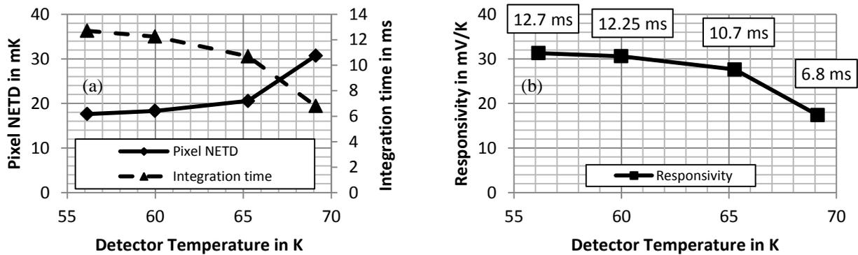
Figure 4. (a) pixel NETD in mK and (b) responsivity in mV/K of the detector for different temperatures
