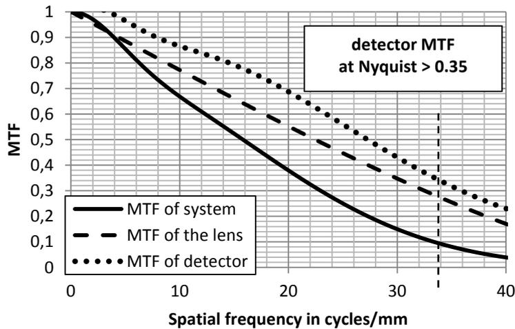
**Figure 11.** MTF of the detector (dotted line) calculated from a MTF measurement on camera level (solid line) and a MTF of a diffraction limited system (dashed line).
