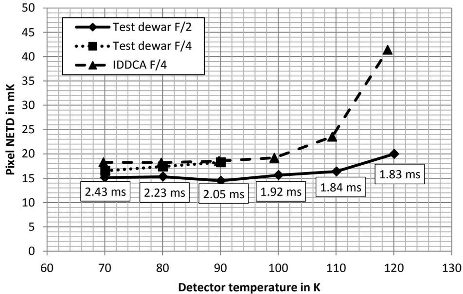
Figure 13. Pixel NETD on IDDCA and test dewar level
